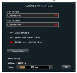
Make sure that the **Sample Rate** here matches the Sample Rate you selected in your DAW and set the desired delay in ms using the slider.
