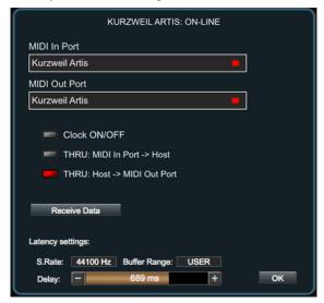
Match with the Buffer Rage size in the Logic's Audio Preferences choosing **Small**, **Medium** or **Large**. You can make further adjustments if you select **User** and set the desired delay in ms using the slider.
