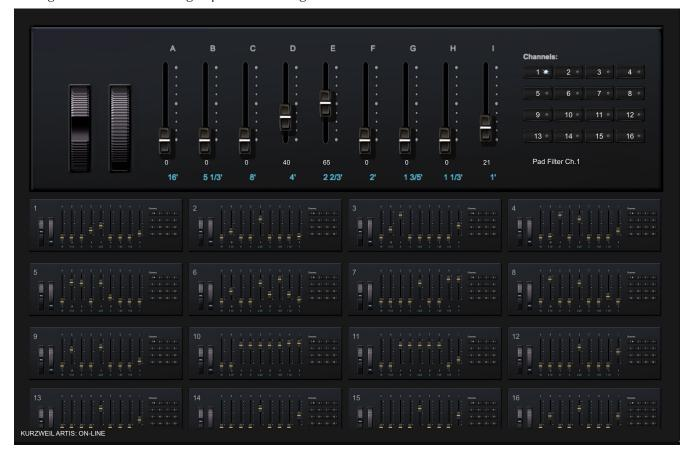
This window emulates the faders and switches on the left side of the Artis® Stage Piano. Moving any of the faders or selecting switches on the Artis® will be seen in the PlugSE<sup>TM</sup> view.
